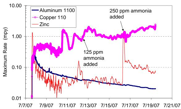
Figure 2 – Effect of Ammonia on Metal Corrosion in Silica Treated Tower Water (without TTA)
