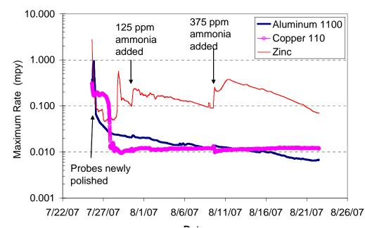
Figure 3 – Effect of Ammonia on Metal Corrosion in Silica Treated Tower Water, with TTA
