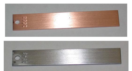
Figure 5 – Copper & Steel Test Coupons, 99 days exposure.
