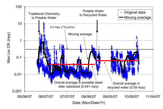
Figure 4 - Real Time CMAS Copper Study, during Change from Potable to Recycled Water.
