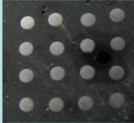
Carbon steel, one week in high-silica brine solution (pH=10) at up to 190 °F
