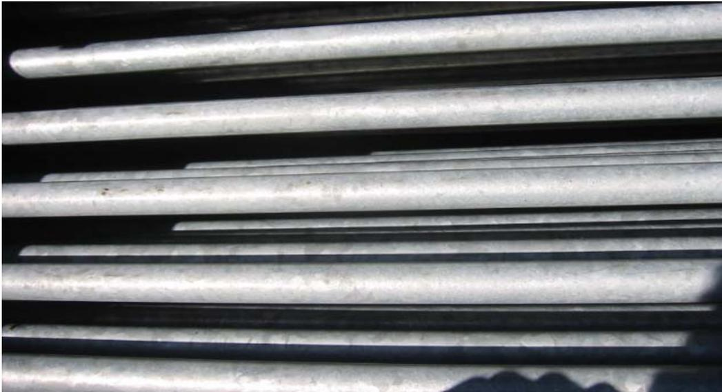
**Figure 5** - # 1652 CS (61 days, 0.017 mpy), # 1664 CS (control, 0.013 mpy)
