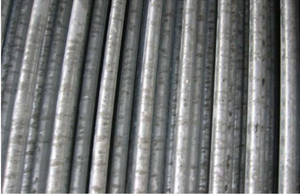
**Figure 4 – EC 10 Galvanized Tubes (20 Months Service)**
