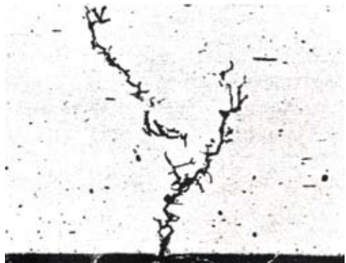
Figure 45. Photomicrograph of intergranular stress corrosion cracking.
