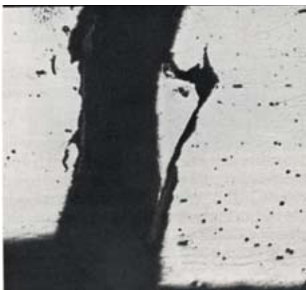
Figure 47. Fatigue crack with stress corrosion cracking emanating from the fracture face.
