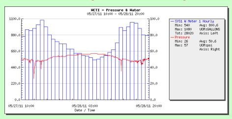
Monitors makeup water usage and water pressure, emails low pressure alarm
