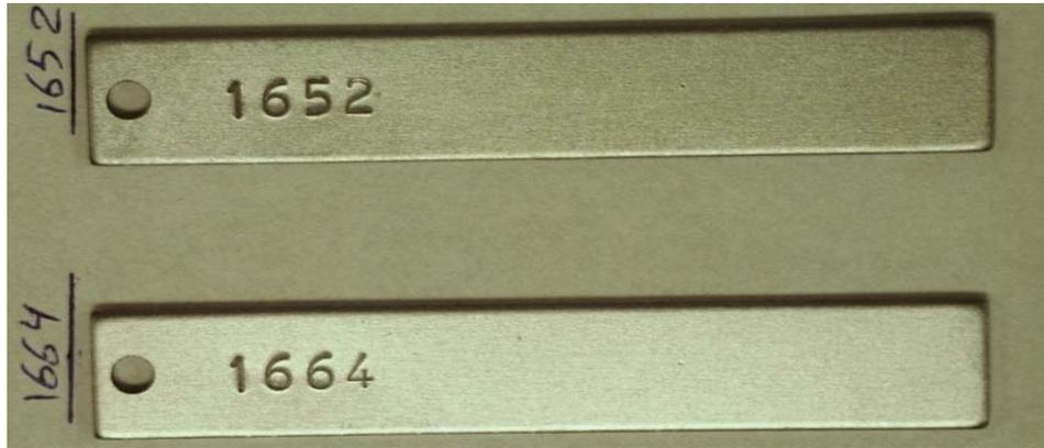
**Figure IV** – Galvanized Coupon # 234 exposed 60 days.
