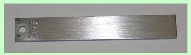
Carbon steel coupon exposed 99 days with 0.426 mpy corrosion rate (high under mount corrosion bias).
