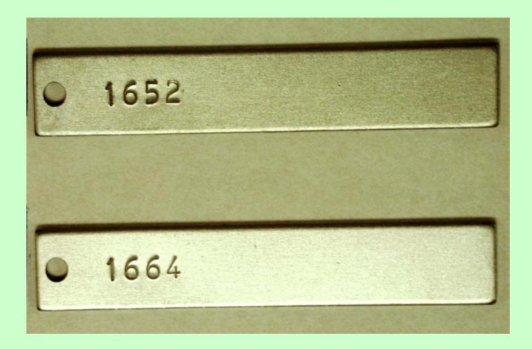
Steel Mill – Galvanized Tubes – 30 Months Service No White Rust at up to 146,000 mg/L TDS Galvanized Coupon after 60 days exposure
