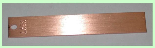
Copper coupon, exposed 99 days, 0.16 mpy corrosion rate (high under mount corrosion bias).
