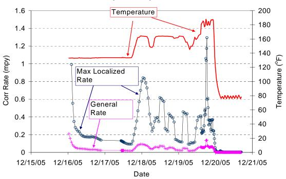
Figure 7 - Localized and General Corrosion Rates of Aluminum 1100 in High Silica / High TDS Water
