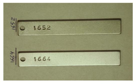
Figure 5 – Bottom # 283 GS exposed 60 days, Top # 282 GS (control)
